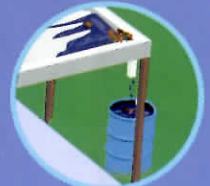
Flat roof without adequate drainage
